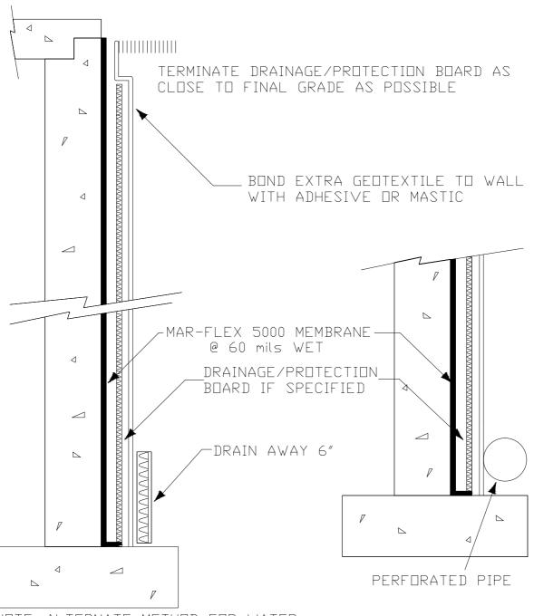
NOTE: ALTERNATE METHOD FOR WATER COLLECTION, SEE DRAIN AWAY FOUNDATION DRAINAGE FOR FITTINGS AND ADAPTORS
